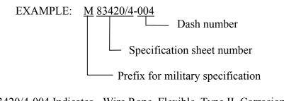
M83420/4-004 Indicates - Wire Rope, Flexible, Type II, Corrosion Resistant Steel, Jacketed, Construction; 7 x 19, Nominal Diameter 3/32, 1/8 Outside Diameter Jacket
