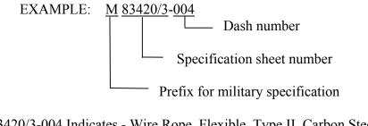
M83420/3-004 Indicates - Wire Rope, Flexible, Type II, Carbon Steel, Construction; 7 x 19, Nominal Diameter 3/16, 1/4 Outside Diameter Jacket
